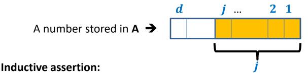
At the end of **jth** iteration, array **A** is sorted according to the last **j** digits.
