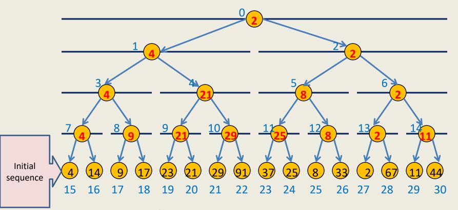
**Data structure:** An array **A** of size 2n-1.
