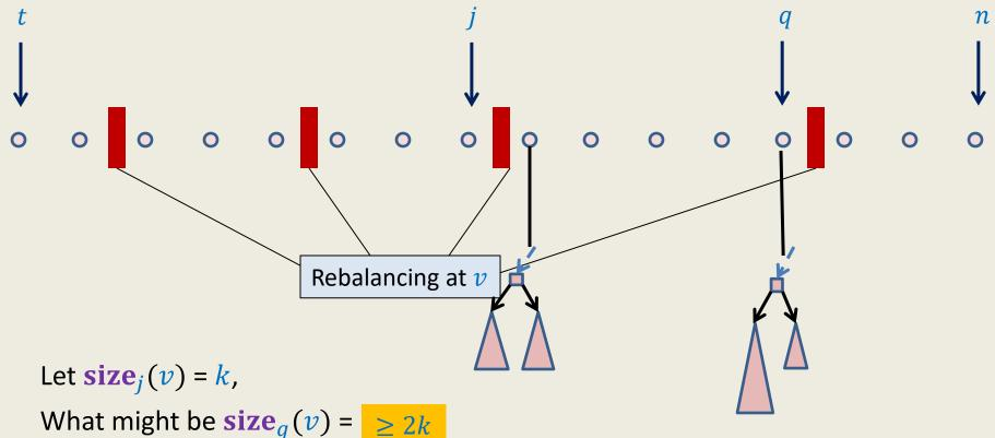
Time complexity of rebalancing T(v) after qth insertion = O(k)
